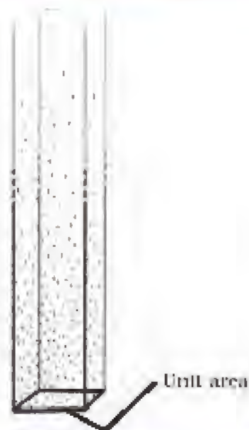
Fig. 9.17 : Atmospheric Pressure is the Weight of Air in a Column of Unit Area
